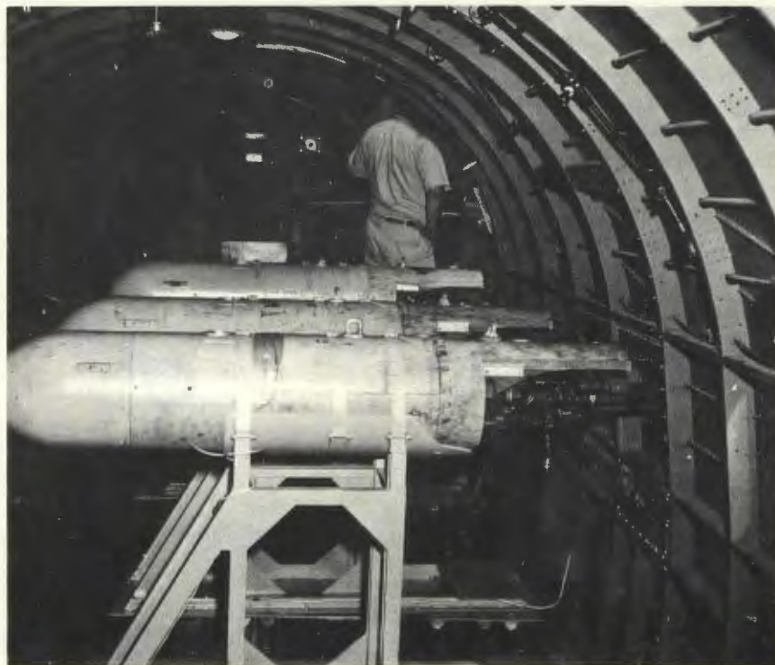
Puff's mini-gun armament is mounted in the fuselage and fired remotely by the pilot.
